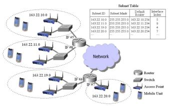
Fig. 2. A WLAN configuration and its subnet table.
