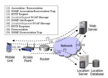
Fig. 3. A web service framework for WLAN location-based services.
