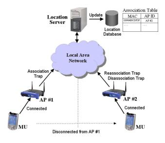
Fig. 1. The SNMP trap approach.
